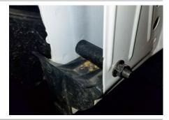
Place the fender back into place and secure using an M6 bolt, lock washer and flat washer.
